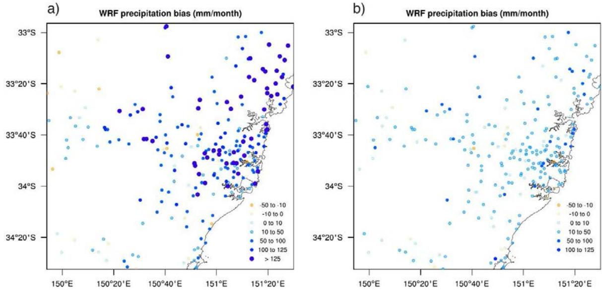
Figure 3 Annual precipitation biases with respect to Bureau of Meteorology stations. a) Non-corrected present-day WRF simulation driven by CSIRO-MK3.5. b) bias-corrected present-day WRF simulation driven by CSIRO-MK3.5.
