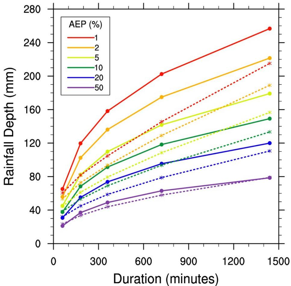
Figure 2 Domain average IFD curves for bias corrected WRF (solid lines) and Bureau of Meteorology observational estimates (dashed lines).
