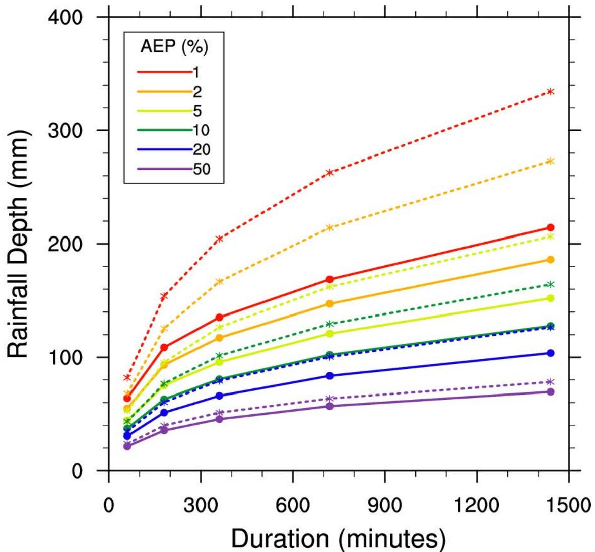
Figure 4 Domain average IFD curves for bias corrected WRF: 1990-2009 (solid lines) and 2040-2059 (dashed lines).
